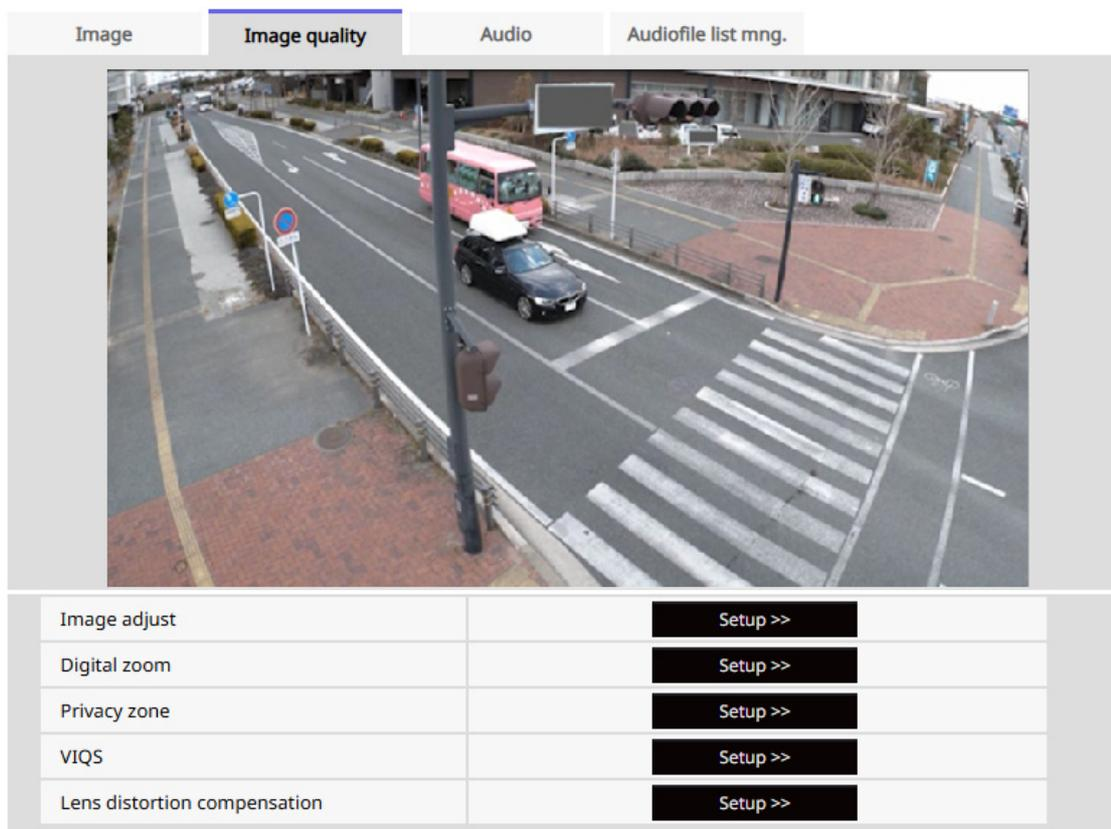
Selecting the camera from the pull-down menu at the bottom of the screen displays the live picture of the selected camera. You can view the image quality adjusted on this screen.
